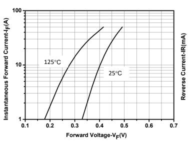
Fig.1-Typical Forward Voltage Characteristics
