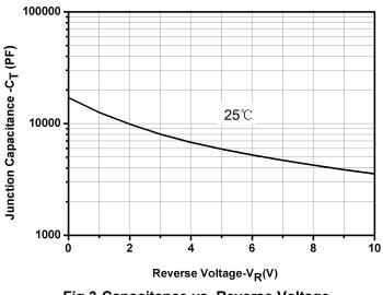
Fig.3-Capacitance vs. Reverse Voltage
