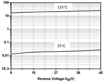
**Fig.2-Typical Reverse Characteristics**
